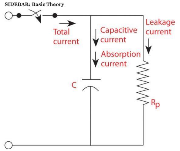
An equivalent circuit for electrical insulation is shown in **Fig. 5** (right). The top terminal might be the center conductor of a power cable, and the bottom terminal, its shield. The current flowing through the cable's insulation would be that current noted as "total current" in the diagram. As you can see, the total current is equal to the sum of the "capacitive current" plus the "leakage current."
