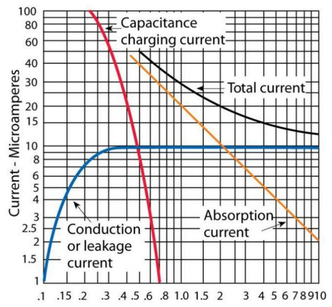
If a DC voltage is suddenly applied (closing the switch in Fig. 5), electrons will rush into the negative plate and be drawn from the positive plate. Initially, this current flow will be very large, but it will gradually reduce to a much smaller value, eventually approaching zero. The
